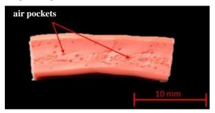
*Figure 9: Parts made of ABS showing interlayer defects* (*Image source: TU-Ilmenau*)
