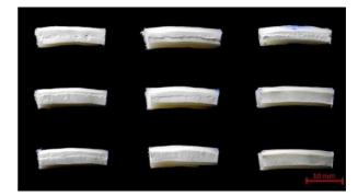
Figure 8: Parts made of ABS showing good bonding quality (Image source: TU-Ilmenau)
